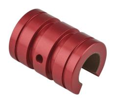
PBC Simplicity series open plain bearing, PTFE, 1/2in inside diameter, 7/8in outside diameter, 1-1/4in overall length, 0.0015in running clearance. For use with 1/2in diameter PBC shafts.
