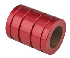
PBC Simplicity series closed plain bearing, PTFE, 1-1/4in inside diameter, 2in outside diameter, 2-5/8in overall length, 0.0015in running clearance. For use with 1-1/4in diameter PBC shafts.
