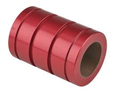
PBC Simplicity series closed plain bearing, PTFE, 1in inside diameter, 1-9/16in outside diameter, 2-1/4in overall length, 0.0015in running clearance. For use with 1in diameter PBC shafts.
