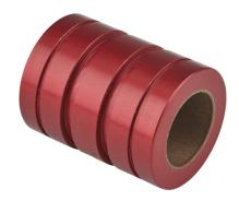
PBC Simplicity series closed plain bearing, PTFE, 3/4in inside diameter, 1-1/4in outside diameter, 1-5/8in overall length, 0.0015in running clearance. For use with 3/4in diameter PBC shafts.
