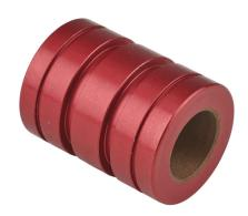
PBC Simplicity series closed plain bearing, PTFE, 5/8in inside diameter, 1-1/8in outside diameter, 1-1/2in overall length, 0.0015in running clearance. For use with 5/8in diameter PBC shafts.
