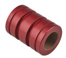
PBC Simplicity series closed plain bearing, PTFE, 1/2in inside diameter, 7/8in outside diameter, 1-1/4in overall length, 0.0015in running clearance. For use with 1/2in diameter PBC shafts.
