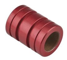
PBC Simplicity series closed plain bearing, PTFE, 3/8in inside diameter, 5/8in outside diameter, 7/8in overall length, 0.0015in running clearance. For use with 3/8in diameter PBC shafts.
