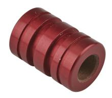
PBC Simplicity series closed plain bearing, PTFE, 1/4in inside diameter, 1/2in outside diameter, 3/4in overall length, 0.0015in running clearance. For use with 1/4in diameter PBC shafts.
