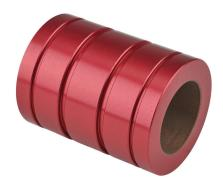
PBC Simplicity series closed plain bearing, PTFE, 1-1/4in inside diameter, 2in outside diameter, 2-5/8in overall length, 0.0005in running clearance. For use with 1-1/4in diameter PBC shafts.
