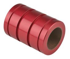
PBC Simplicity series closed plain bearing, PTFE, 1in inside diameter, 1-9/16in outside diameter, 2-1/4in overall length, 0.0005in running clearance. For use with 1in diameter PBC shafts.
