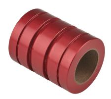
PBC Simplicity series closed plain bearing, PTFE, 3/4in inside diameter, 1-1/4in outside diameter, 1-5/8in overall length, 0.0005in running clearance. For use with 3/4in diameter PBC shafts.
