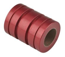
PBC Simplicity series closed plain bearing, PTFE, 5/8in inside diameter, 1-1/8in outside diameter, 1-1/2in overall length, 0.0005in running clearance. For use with 5/8in diameter PBC shafts.
