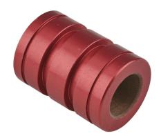
PBC Simplicity series closed plain bearing, PTFE, 1/2in inside diameter, 7/8in outside diameter, 1-1/4in overall length, 0.0005in running clearance. For use with 1/2in diameter PBC shafts.
