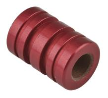
PBC Simplicity series closed plain bearing, PTFE, 1/4in inside diameter, 1/2in outside diameter, 3/4in overall length, 0.0005in running clearance. For use with 1/4in diameter PBC shafts.
