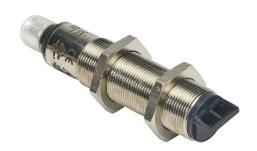
AchieVe photoelectric sensor, tubular, threaded, diffuse with background suppression, 90-degree, 30-130mm sensing distance, complementary light-on/dark-on, PNP, potentiometer, 1.5 kHz switching frequency, 4-pin M12 quick-disconnect.
