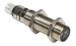
AchieVe photoelectric sensor, tubular, threaded, diffuse with background suppression, 30-150mm sensing distance, complementary light-on/dark-on, PNP, potentiometer, 1.5 kHz switching frequency, 4-pin M12 quick-disconnect.
