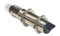
AchieVe photoelectric sensor, tubular, threaded, diffuse with background suppression, 90-degree, 30-130mm sensing distance, complementary light-on/dark-on, NPN, potentiometer, 1.5 kHz switching frequency, 4-pin M12 quick-disconnect.
