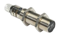
AchieVe photoelectric sensor, tubular, threaded, diffuse with background suppression, 30-150mm sensing distance, complementary light-on/dark-on, NPN, potentiometer, 1.5 kHz switching frequency, 4-pin M12 quick-disconnect.
