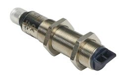
AchieVe photoelectric sensor, tubular, threaded, diffuse with background suppression, 90-degree, 30-80mm sensing distance, complementary light-on/dark-on, PNP, potentiometer, 1.5 kHz switching frequency, 4-pin M12 quick-disconnect.
