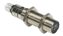
AchieVe photoelectric sensor, tubular, threaded, diffuse with background suppression, 30-100mm sensing distance, complementary light-on/dark-on, PNP, potentiometer, 1.5 kHz switching frequency, 4-pin M12 quick-disconnect.
