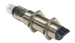
AchieVe photoelectric sensor, tubular, threaded, diffuse with background suppression, 90-degree, 30-80mm sensing distance, complementary light-on/dark-on, NPN, potentiometer, 1.5 kHz switching frequency, 4-pin M12 quick-disconnect.
