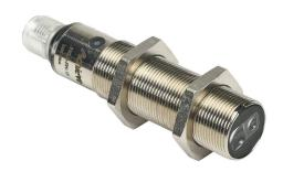
AchieVe photoelectric sensor, tubular, threaded, diffuse with background suppression, 30-100mm sensing distance, complementary light-on/dark-on, NPN, potentiometer, 1.5 kHz switching frequency, 4-pin M12 quick-disconnect.
