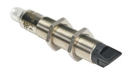
AchieVe photoelectric sensor, tubular, threaded, polarized retroreflective, 90-degree, Class 1 red laser, 0.05-30m sensing distance, complementary light-on/dark-on, PNP, teach-in button, 4-wire, 4-pin M12 quick-disconnect.
