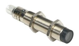
AchieVe photoelectric sensor, tubular, threaded, polarized retroreflective, Class 1 red laser, 0.05-30m sensing distance, complementary light-on/dark-on, PNP, teach-in button, 4-wire, 4-pin M12 quick-disconnect.
