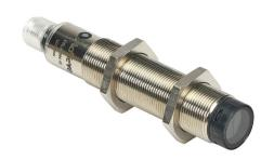
AchieVe photoelectric sensor, tubular, threaded, polarized retroreflective, Class 1 red laser, 0.05-30m sensing distance, complementary light-on/dark-on, NPN, teach-in button, 4-wire, 4-pin M12 quick-disconnect.
