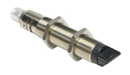
AchieVe photoelectric sensor, tubular, threaded, nickel-plated brass housing, through-beam emitter, 90-degree, Class 1 red laser, 0.05-50m sensing distance, 10-30 VDC operating voltage, 3-wire, 4-pin M12 quick-disconnect.
