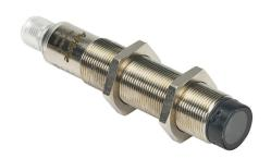
AchieVe photoelectric sensor, tubular, threaded, nickel-plated brass housing, through-beam emitter, Class 1 red laser, 0.05-50m sensing distance, 10-30 VDC operating voltage, 3-wire, 4-pin M12 quick-disconnect.
