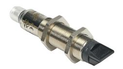
AchieVe photoelectric sensor, tubular, threaded, nickel-plated brass housing, through-beam receiver, 90-degree, 0.05-50m sensing distance, 10-30 VDC operating voltage, complementary light-on/dark-on, PNP, 4-wire, 4-pin M12 quick-disconnect.
