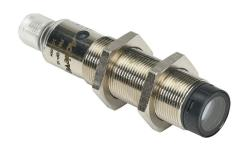
AchieVe photoelectric sensor, tubular, threaded, nickel-plated brass housing, through-beam receiver, 0.05-50m sensing distance, 10-30 VDC operating voltage, complementary light-on/dark-on, PNP, 4-wire, 4-pin M12 quick-disconnect.
