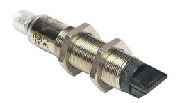
AchieVe photoelectric sensor, tubular, threaded, nickel-plated brass housing, through-beam receiver, 90-degree, 0.05-50m sensing distance, 10-30 VDC operating voltage, complementary light-on/dark-on, NPN, 4-wire, 4-pin M12 quick-disconnect.
