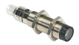
AchieVe photoelectric sensor, tubular, threaded, nickel-plated brass housing, through-beam receiver, 0.05-50m sensing distance, 10-30 VDC operating voltage, complementary light-on/dark-on, NPN, 4-wire, 4-pin M12 quick-disconnect.
