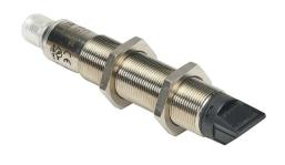
AchieVe photoelectric sensor, tubular, threaded, diffuse, 90-degree, Class 1 red laser, 0-200mm sensing distance, complementary light-on/dark-on, PNP, 1 kHz switching frequency, teach-in button, nickel-plated brass housing, 4-pin M12 quick-disconnect.
