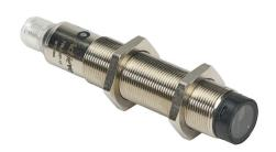
AchieVe photoelectric sensor, tubular, threaded, diffuse, Class 1 red laser, 0-300mm sensing distance, complementary light-on/dark-on, PNP, teach-in button, 1 kHz switching frequency, nickel-plated brass housing, 4-pin M12 quick-disconnect.
