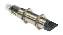
AchieVe photoelectric sensor, tubular, threaded, diffuse, 90-degree, Class 1 red laser, 0-200mm sensing distance, complementary light-on/dark-on, NPN, 1 kHz switching frequency, teach-in button, nickel-plated brass housing, 4-pin M12 quick-disconnect.
