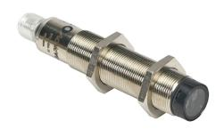
AchieVe photoelectric sensor, tubular, threaded, diffuse, Class 1 red laser, 0-300mm sensing distance, complementary light-on/dark-on, NPN, teach-in button, 1 kHz switching frequency, nickel-plated brass housing, 4-pin M12 quick-disconnect.
