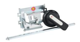
Eaton rotary handle, pistol, black, external front mount, 2-position, lockable in OFF only, defeatable, NEMA 1/12. For use with AutomationDirect (Eaton) 225A frame MCCBs. 12in shaft and operator included.
