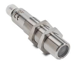
AutomationDirect photoelectric sensor, tubular, threaded, 316L stainless steel, diffuse with background suppression, 30-130mm sensing distance, complementary light-on/dark-on, PNP, teach-in button, 1 kHz switching frequency, 4-pin M12 quick-disconnect.
