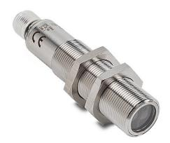
AutomationDirect photoelectric sensor, tubular, threaded, 316L stainless steel, diffuse with background suppression, 30-130mm sensing distance, complementary light-on/dark-on, NPN, teach-in button, 1 kHz switching frequency, 4-pin M12 quick-disconnect.
