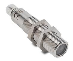
AutomationDirect photoelectric sensor, tubular, threaded, 316L stainless steel, diffuse with background suppression, 60-100mm sensing distance, complementary light-on/dark-on, NPN, teach-in button, 400 Hz switching frequency, 4-pin M12 quick-disconnect.
