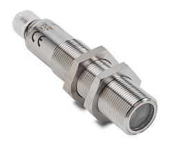
AutomationDirect photoelectric sensor, tubular, threaded, 316L stainless steel, diffuse with background suppression, 60-100mm sensing distance, selectable light-on/dark-on, PNP, teach-in button, 400 Hz switching frequency, 4-pin M12 quick-disconnect.
