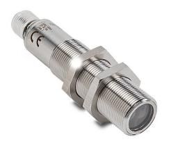
AutomationDirect photoelectric sensor, tubular, threaded, 316L stainless steel, diffuse with background suppression, 30-130mm sensing distance, selectable light-on/dark-on, NPN, teach-in button, 1 kHz switching frequency, 4-pin M12 quick-disconnect.
