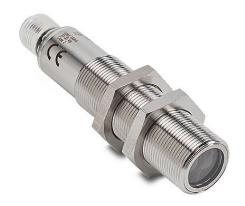
AutomationDirect photoelectric sensor, tubular, threaded, 316L stainless steel, diffuse with background suppression, 60-100mm sensing distance, selectable light-on/dark-on, NPN, teach-in button, 400 Hz switching frequency, 4-pin M12 quick-disconnect.
