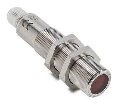
AutomationDirect photoelectric sensor, tubular, threaded, polarized retroreflective, visible red, 4m sensing distance, complementary light-on/dark-on, PNP, 4-wire, 4-pin M12 quickdisconnect.
