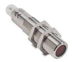
AutomationDirect photoelectric sensor, tubular, threaded, polarized retroreflective, visible red light emission, 4m sensing distance, complementary light-on/dark-on, PNP, 4-wire, 4-pin M12 quick-disconnect.
