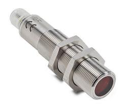
AutomationDirect photoelectric sensor, tubular, threaded, polarized retroreflective, visible red light emission, 4m sensing distance, complementary light-on/dark-on, NPN, 4-wire, 4-pin M12 quick-disconnect.
