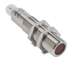
AutomationDirect photoelectric sensor, tubular, threaded, polarized retroreflective, visible red, 4m sensing distance, selectable light-on/dark-on, PNP, 4-wire, 4-pin M12 quick-disconnect.
