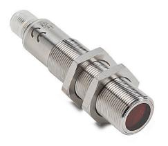
AutomationDirect photoelectric sensor, tubular, threaded, polarized retroreflective, visible red, 4m sensing distance, selectable light-on/dark-on, NPN, 4-wire, 4-pin M12 quick-disconnect.
