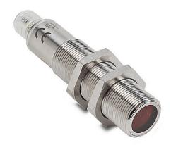
AutomationDirect photoelectric sensor, tubular, threaded, polarized retroreflective, visible red, 4m sensing distance, complementary light-on/dark-on, PNP, teach-in button, 4-wire, 4-pin M12 quick-disconnect.
