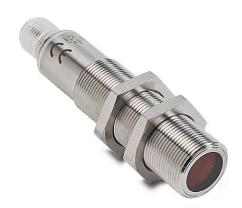
AutomationDirect photoelectric sensor, tubular, threaded, polarized retroreflective, visible red, 4m sensing distance, complementary light-on/dark-on, NPN, teach-in button, 4-wire, 4-pin M12 quick-disconnect.
