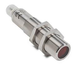
AutomationDirect photoelectric sensor, tubular, threaded, polarized retroreflective, visible red, 4m sensing distance, selectable light-on/dark-on, PNP, teach-in button, 4-wire, 4-pin M12 quick-disconnect.
