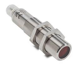
AutomationDirect photoelectric sensor, tubular, threaded, polarized retroreflective, visible red, 4m sensing distance, selectable light-on/dark-on, NPN, teach-in button, 4-wire, 4-pin M12 quick-disconnect.
